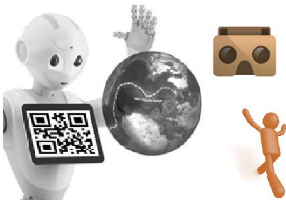
Fig.1: Using Pepper Robot's Built-in Tablet and AR Headset for Providing Augmented Reality
