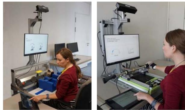
**Figure 1:** First prototype of telerehabilitation systems based on haptic therapeutic devices Bi-Manu-Track (left) and Reha-Slide (right).
